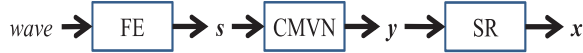
Figure 1. Block diagram of our TMSR processing technique. Abbreviations stand for: FE - feature extraction; CMVN - conventional CMVN process; SR - spectral restoration.
