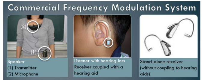
Fig. 1. Conventional FM system with a transmitter–receiver pair. The speaker wears the transmitter (left, [13]), and the listener with HL wears the receiver for listening. The receiver can be coupled with a hearing aid (middle, [13]) or standalone (right, http://www.phonak.com ).
